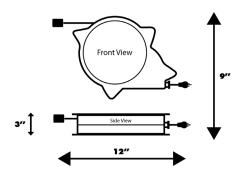
Dimensions – 9" x 12" x 3" Molded Polypropylene 3.175 mm Thickness 94V-0 Flammability Rating
